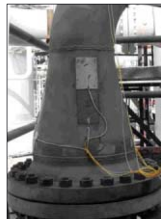
Fig. 1a (left) shows a general view of the selected 20-in. x 12-in. reducer; Fig. 1b shows the fiber-optic sensors attached on the reducer.
